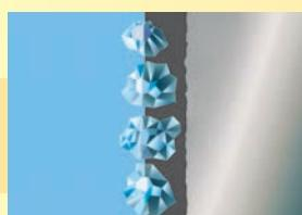
Diamond crystals in an electro-deposited metal bond.
