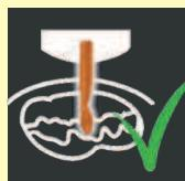
Thanks to a special cutting geometry, it is also possible to take thermoplastic materials, which have properties which allow them to spread quickly and clog up the tool, and mill them without water cooling.
