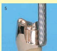
After casting and finishing of the crown, the parallel surface is remilled with the profile bur F137 3H 23.
