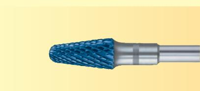
The diatit titanium burs have a special cross cut, which enlarges the chip space and therefore reduces friction when titanium processing. Overheating of the titanium is thereby avoided.
