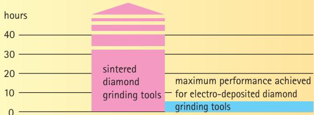
Summary: When comparing sintered/electroplated diamond grinding tools in the long-term test, the bredient Diabolo tools excelled due to their efficiency and extended service life. Thanks to the self-sharpening properties of the diamond crystals, the sintered diamond tools feature high cutting performance and ensure perfect removal of material for the duration of service life.
