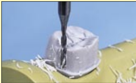
Excellent milling of wax due to variably adjustable speed.
