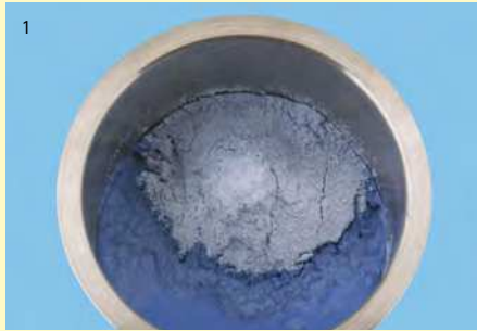
1 Mix Fluid-Rock base stone in the ratio of 100 g powder and 25 ml distilled water to achieve a highly fluid consistency.
