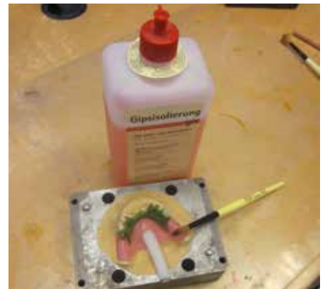
All undercut areas must be sealed off with plaster to ensure that the flask halves open correctly.
