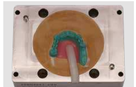
Film sprue of a UK telescope injection-moulded base.
