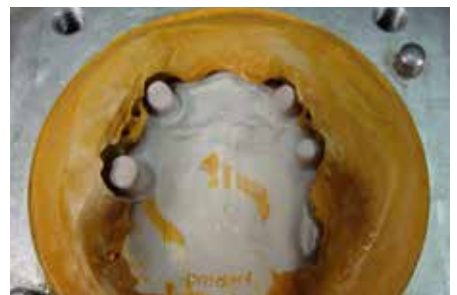
After the wax model has been boiled out, the plaster and wax residues can be removed with a soft toothbrush and washing-up liquid. Insulate the model with Acrylic Sep directly when it is still warm from the boiling water.
