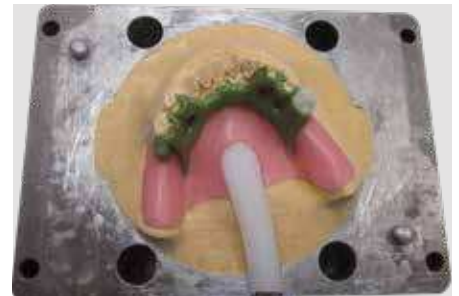
Spruing with 2 sprue channels.
