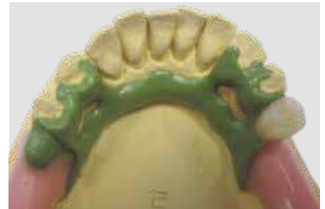
Wax modelling of an attachment model injection moulding base with pink plate wax.
