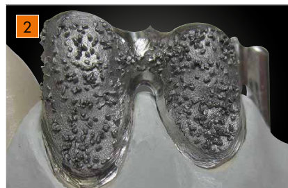
Completed crown framework.
