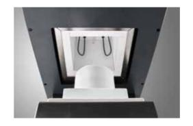
High-quality molybdenum disilicide heating elements reach a maximum end temperature of 1.650°C. Unlike silicon carbide heating systems, heaters of this type are far enough away from their maximum performance limit of approx. 1.800°C. Thanks to this property they attain a significantly longer service life. Each of the four heating elements can be individually replaced in case of damage – an "en bloc" replacement is unnecessary.
