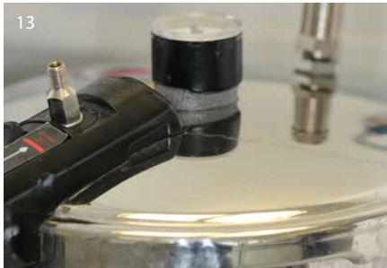
13 Pressure pot, 3-4 bar, approx. 50°C, 10 minutes.
