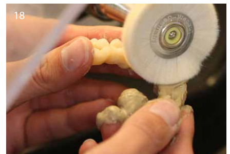
18 Remove excess Qu-resin dentin and finish. Polish with goat-hair brush and cotton buff. If required, repolish with handpiece and Acrypol. Above all, basal areas need to be polished thoroughly.
