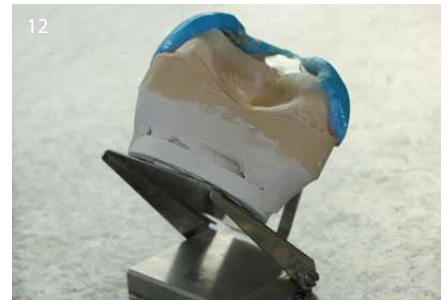
12 Posi-boy is used for accurate positioning.
