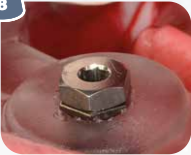
The exact coverage of the two hexagons is important for the exact position of the RevoCone base.
